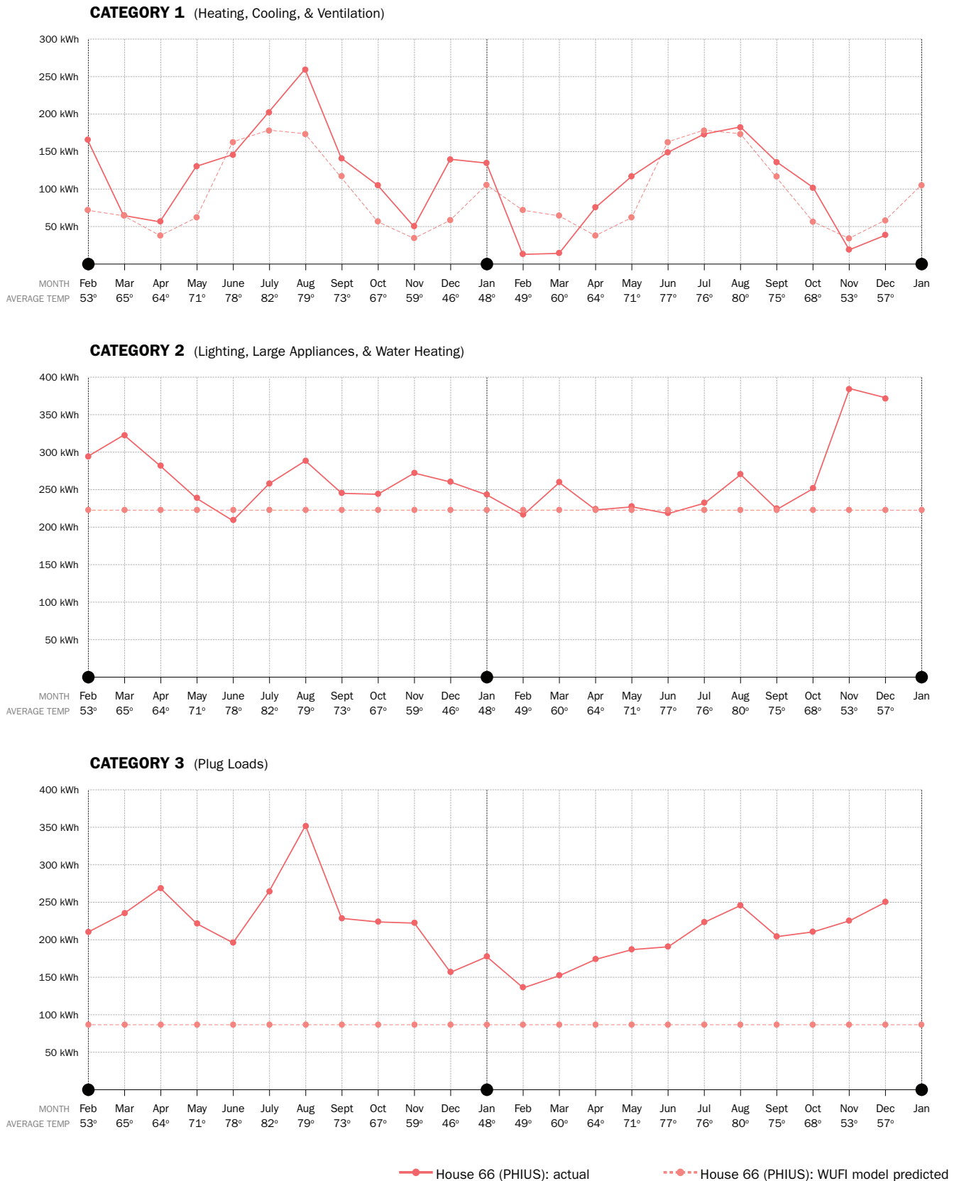
Figure 5. Comparison of modeled and actual energy use in Categories 1,2, and 3 at House 66. Image credit Auburn University.
